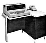
Multics. Built into a desk with a desk-side box for the electronics. It had a row of switches above the keyboard for doing things like controlling the paper tape reader. Used a device dependent 6-bit character set related to BCD, but with shift codes to access the larger character set. This was the first terminal used for serious word processing, because it provided high quality upper and lower case output. Transmission speed was 134.5 baud.
